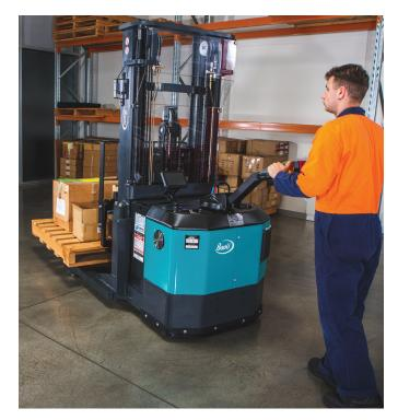
Centrally mounted tiller for excellent visibility of the load
