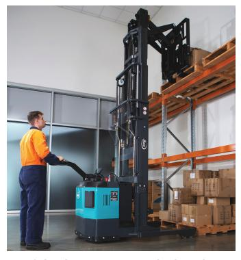
Lift loads over 5 meters high with a reach of almost 600mm
