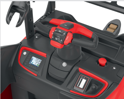
Ergonomic, height-adjustable tiller
