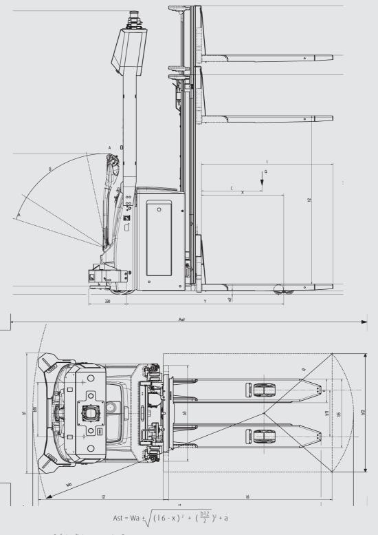
Safety distance a=a1+a2 a1: Front safety distance a2: Rear safety distance
