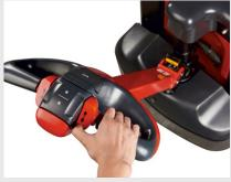
All controls ergonomically integrated in the Linde tiller
