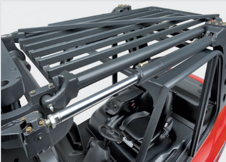
Protective overhead guard
